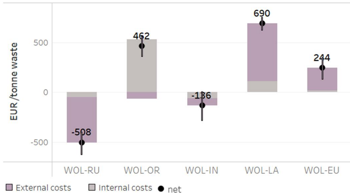
Figure 36. Full environmental life cycle costs for the management of 1 tonne of wool waste (WOL) via re-use (RU), open-loop recycling (OR: production of secondary wipers), incineration (IN) and landfilling (LA) as well as combination of the two last ones according to the EU average management of residual mixed (not separately collected) municipal waste (EU). The error bar represents \pm the standard deviation around the default value. It is referred to Table 7 for a description of the different treatment scenarios and technologies.
