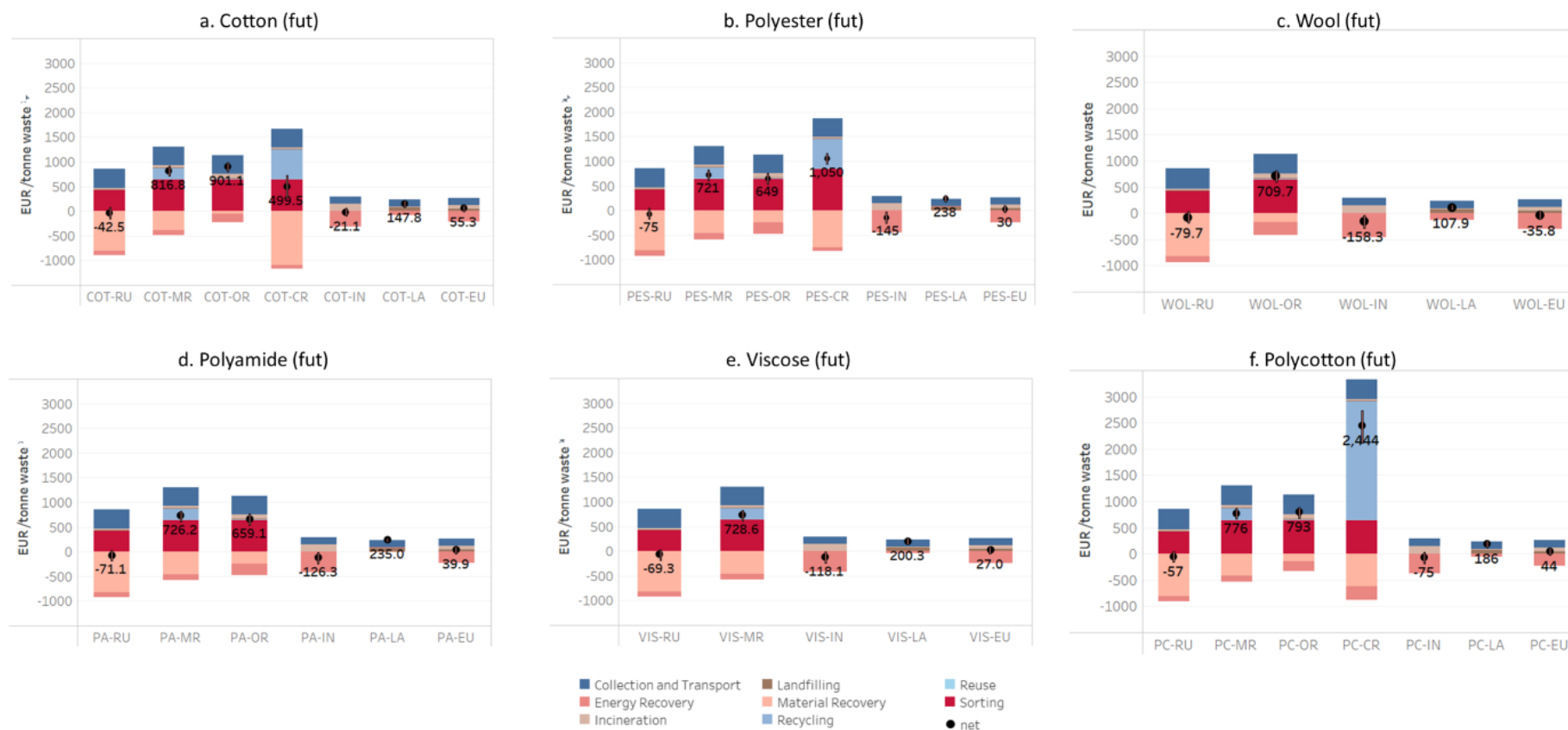
Figure 41. Future scenario analysis - Environmental life cycle costs for the management of 1 tonne of cotton (COT), polyester (PES), wool (WOL), polyamide (PA), viscose (VIS) and polycotton (PC) waste via re-use (RU), mechanical recycling (MR), open-loop recycling (OR), chemical recycling (CR), enzymatic recycling (EN), incineration (IN) and landfilling (LA) as well as combination of the two last ones according to the EU average management of residual mixed (not separately collected) municipal waste (EU). The error bar represents \pm the standard deviation around the default value. It is referred to Table 7 for a description of the different treatment scenarios and technologies. Note that for polycotton, dissolution of polyester and recovery of cotton (PC-CR*, EUR 5 577) and enzymatic recycling (PC-EN, EUR 61 235) are not represented in the Figure because out of scale.
