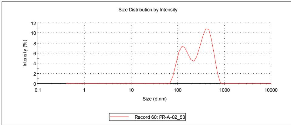
**Figure 23. DLS size distribution by intensity for NM-200 dispersed in Milli-Q<sup>®</sup> water. Pdl = 0.529, peak 1 = 143 nm, peak 2 = 411 nm.**
