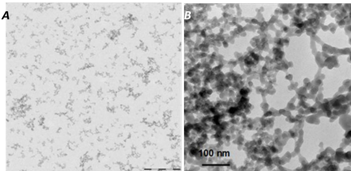
**Figure 55. NM-202: A) Representative TEM micrograph of well-dispersed sample taken for quantitative TEM-analysis; scale bar is 500nm. B) TEM micrograph showing the complex open network structure in the silicon dioxide aggregates; scale bar is 100nm.**
