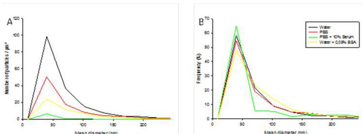
Figure 47. Effect of medium on the size distribution of NM-200. The number of particles per  $\mu\text{m}^2$  of grid area for a concentration of 0.512 mg/ml (A) and corresponding frequencies (B) are represented as a function of their mean diameter.
