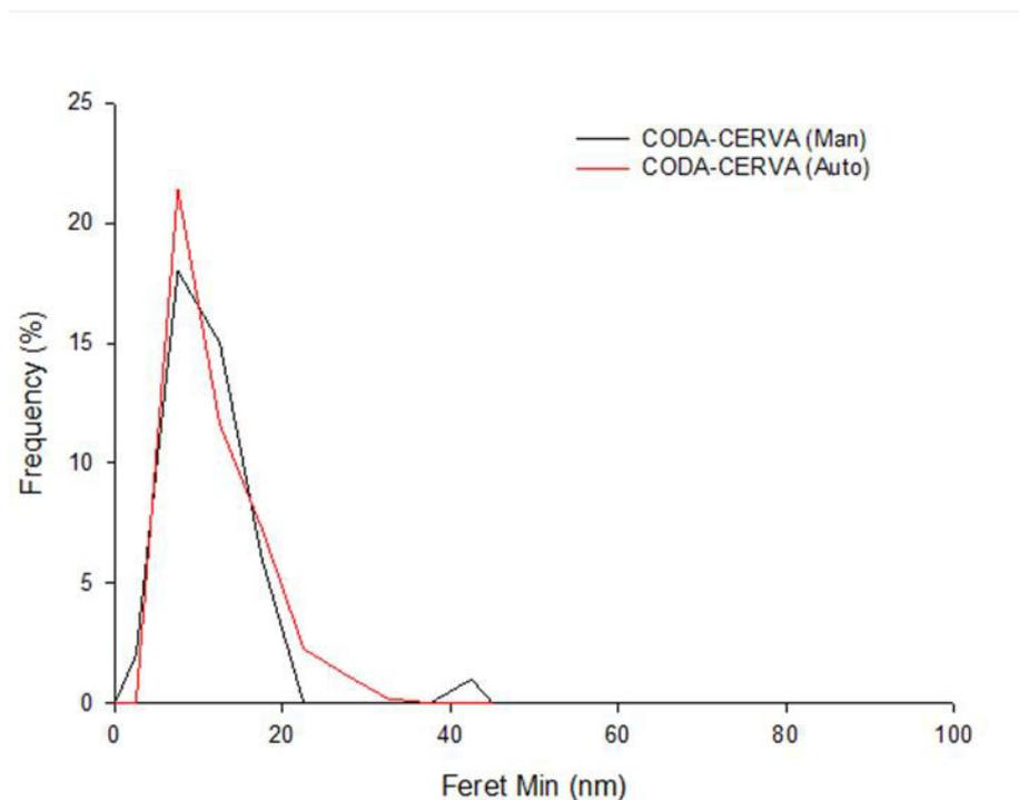
**Figure 59. Qualitative TEM image analysis of NM-203 illustrating the primary particle Feret Min size distribution as a function of the frequency. The manual (CODA-CERVA (Man)) and semi-automatic measurements (CODA-CERVA (Auto)) are given.**
