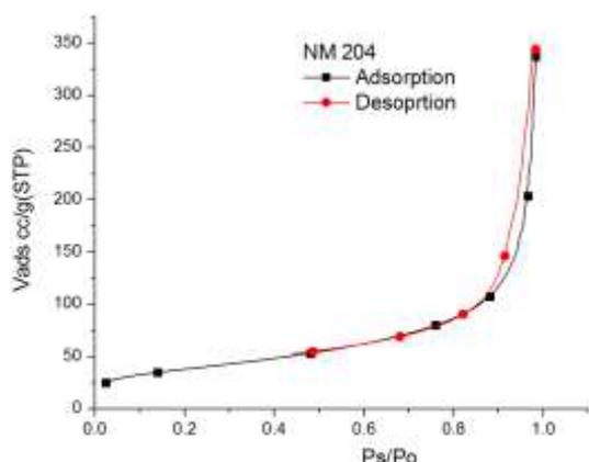
**Figure 37. Isotherms of nitrogen sorption experiments by IMC-BAS at 77K for SAS NMs giving the adsorbed volume (Vads) in cm<sup>3</sup> per gram (cc/g) [y-axis] and P/P<sub>0</sub> on the x-axis. The NM-numbers are mentioned in the title of each plot.**
