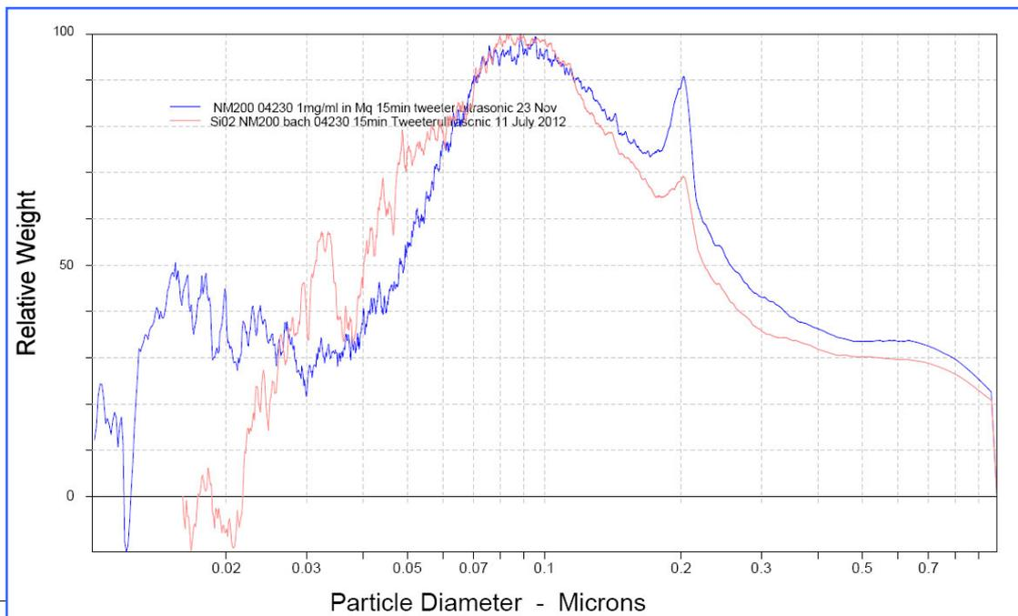
Figure 27. CLS particle size distribution graph for NM-200.
