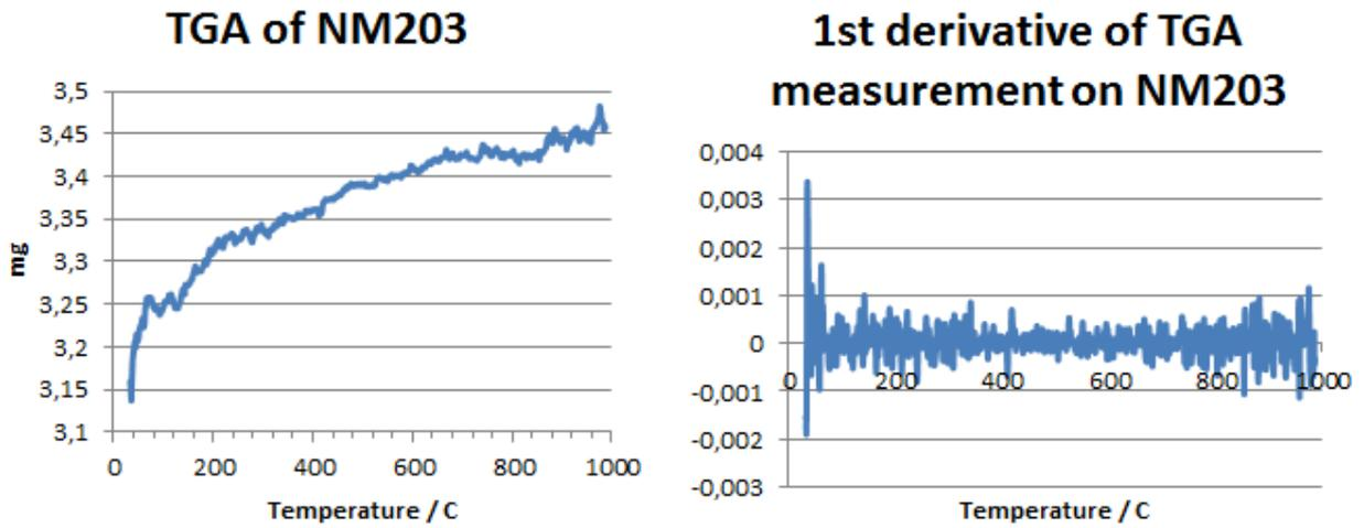
Figure 5. Results from TGA measurement on NM-203. The weight change is due to buoyancy<sup>3</sup>.
