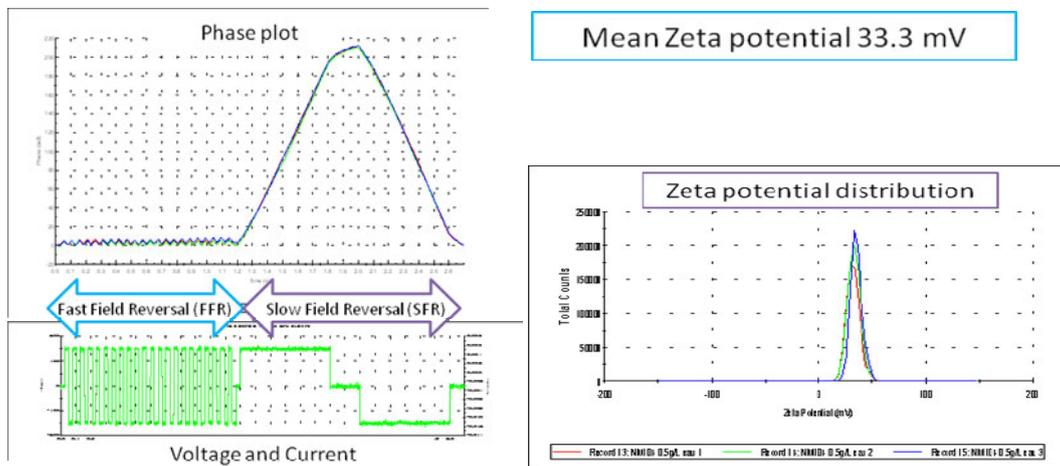
**Figure C3. Data plots retrieved from zeta potential measurements on Nanosizer ZS, example of 3 consecutive measurements on a suspension of NM-104 (TiO<sub>2</sub>) at 0.5 g/L in pure water.**
