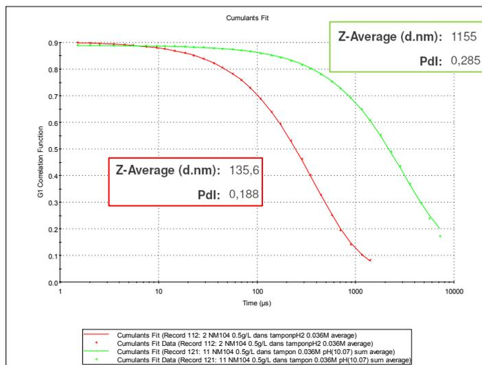
**Figure A6. Example of data and fits by the Cumulant method, together with calculated values of Z average and polydispersity, for two NM-104 (TiO<sub>2</sub>) samples (0.5 g/L TiO<sub>2</sub> in 0.036 mol/L ionic buffer, stable suspension at pH2.8 in red and unstable sample of big aggregates at pH10.1 in green).**
