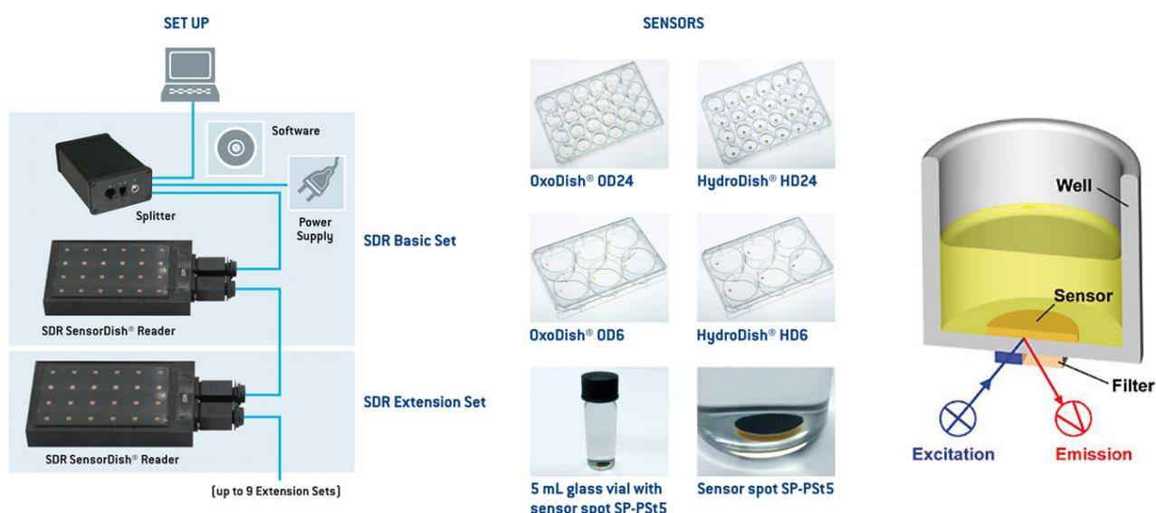
**Figure B1. Sensor Dish Reader, examples of sensor products and illustration of the SDR measurement principle. In this study we used the 24-well Oxy- and HydroDish for O<sub>2</sub> and pH monitoring. Source: PreSens Precision Sensing GmbH, Germany.**
