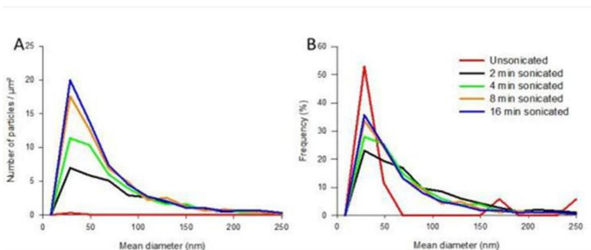
**Figure 45. Effect of sonication on the size distribution of NM-201 (precipitated). The number of particles per  $\mu\text{m}^2$  of grid area for a concentration of 0.512 mg/ml (A) and the corresponding frequencies (B) are represented as a function of their mean diameter.**
