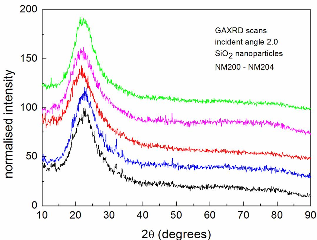
Figure 42. JRC XRD of NM-200 to 204, amorphous. Black: NM-200, blue: NM-201, red: NM-202, pink: NM-203, green: NM-204.
