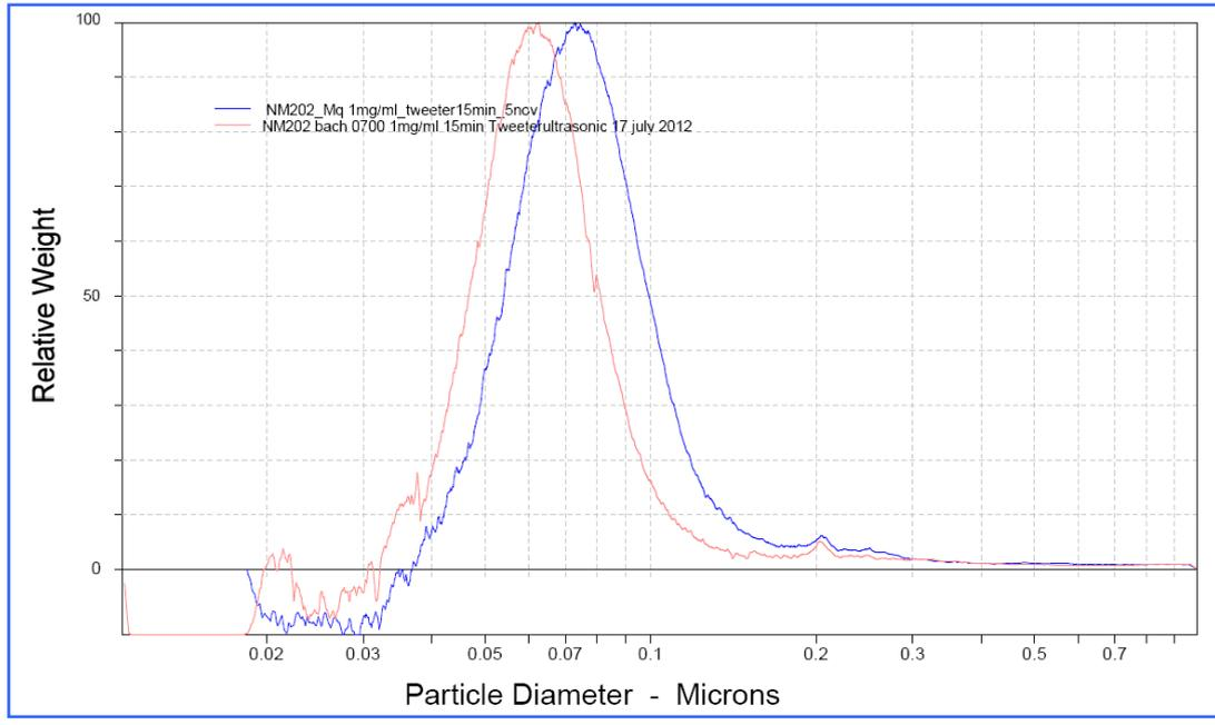
**Figure 29. CLS particle size distribution graph for NM-202.**
