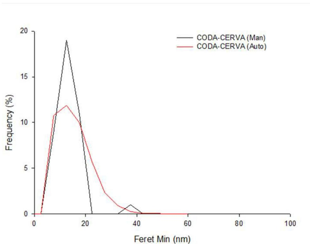
**Figure 53. Qualitative TEM image analysis of NM-201. The graph illustrates the primary particle Feret Min size distribution as a function of the frequency. The manual (CODA-CERVA (Man)) and semi-automatic measurement (CODA-CERVA (Auto)) are given.**
