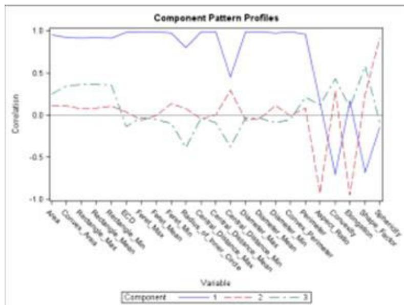
Figure 63 Representative examples of component pattern profiles of quantitative TEM analysis of NM-202 (A) categorized into three principle components (blue line, red dashed line and green dashed line).
