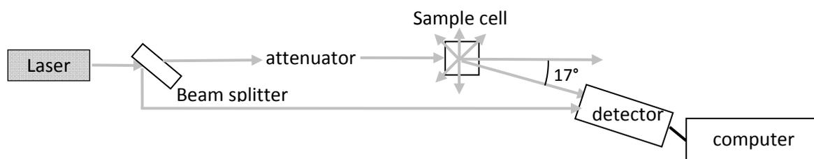
**Figure C2. Simplified scheme of optical configuration for zeta potential measurement on Zetasizer NanoZS.**
