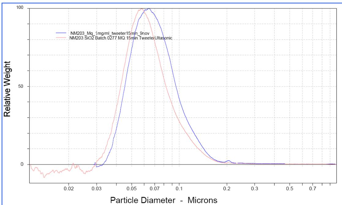
**Figure 30. CLS particle size distribution graph for NM-203.**
