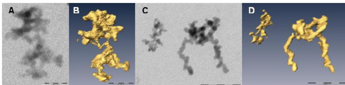
**Figure 65.** Electron tomographic analyses of NM-200 and NM-203. The micrographs, taken at 0°, show one (Figure 65A) and two aggregates (Figure 65C) consisting of multiple primary subunits of NM-200 and NM-203, respectively. Figure 65B and Figure 65D show the corresponding ET reconstructions. Bars: 200 nm.
