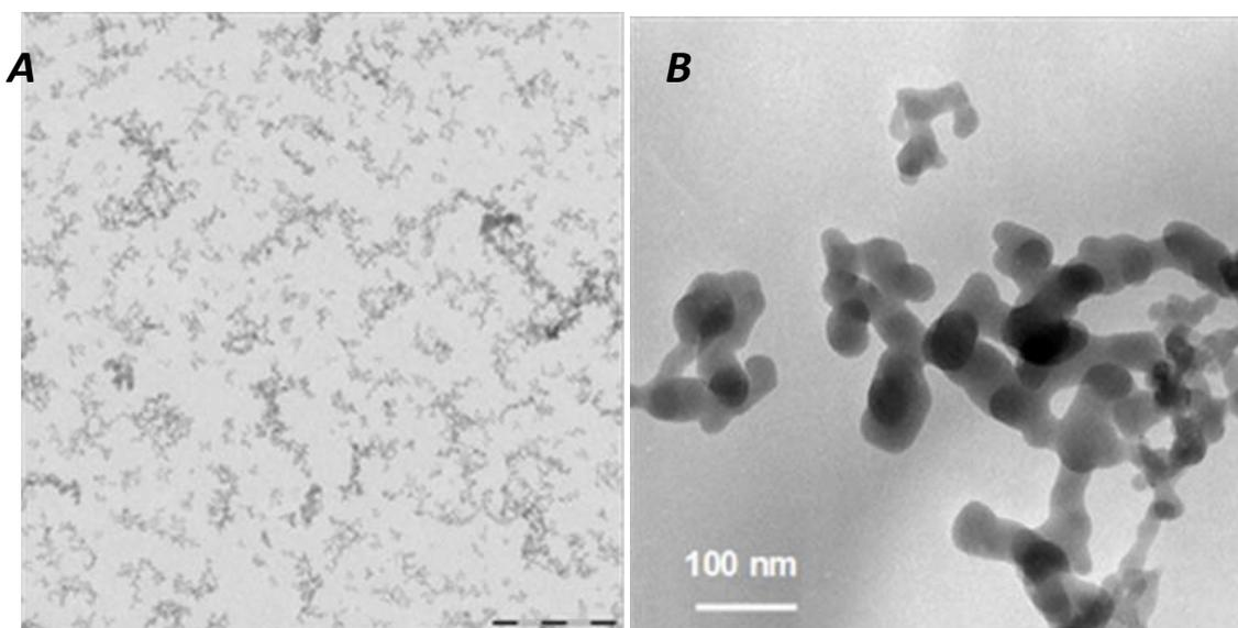
**Figure 58.** NM-203: A) Representative TEM micrograph of well-dispersed sample taken for quantitative TEM-analysis; scale bar is 500nm. B) TEM micrograph showing the complex open network structure in the silicon dioxide aggregates; scale bar is 100nm.
