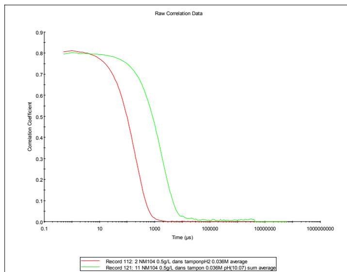
**Figure A5.** Example of raw correlation data for two NM104 samples (0.5 g/L  $\text{TiO}_2$  in 0.036 mol/L ionic buffer), one stable suspension of relatively dispersed particles at pH2.8 (red curve), and one unstable sample of big aggregates at pH10.1 (green curve, measure on supernatant).
