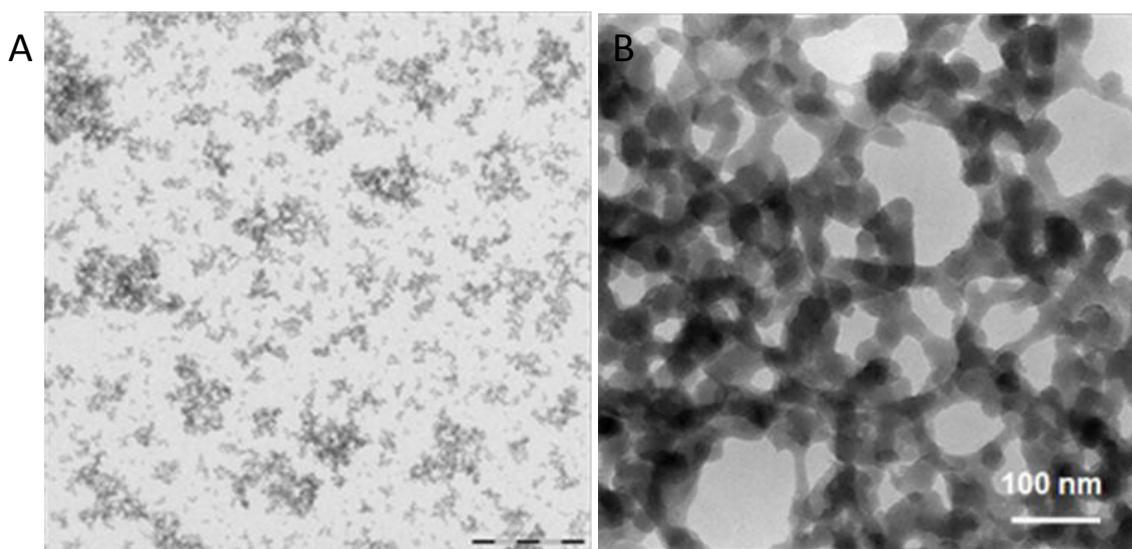
**Figure 52. NM-201: A) Representative TEM micrograph of well-dispersed sample taken for quantitative TEM-analysis; scale bar is 500nm. B) TEM micrograph showing the complex open network structure in the silicon dioxide aggregates; scale bar is 100nm.**
