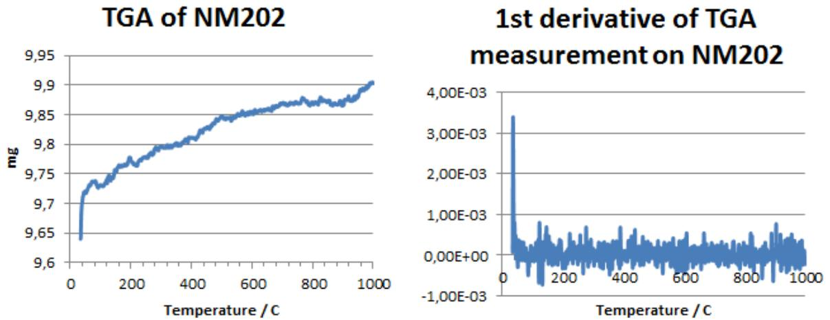
Figure 3. Results from TGA measurement on NM-202. The change in weight is due to buoyancy<sup>3</sup>.
