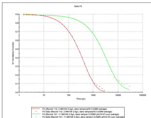
**Figure A7. Example of data and fits by the CONTIN method, for two NM-104 (TiO<sub>2</sub>) samples (0.5 g/L TiO<sub>2</sub> in 0.036 mol/L ionic buffer, stable suspension at pH2.8 in red and unstable sample of big aggregates at pH10.1 in green).**
