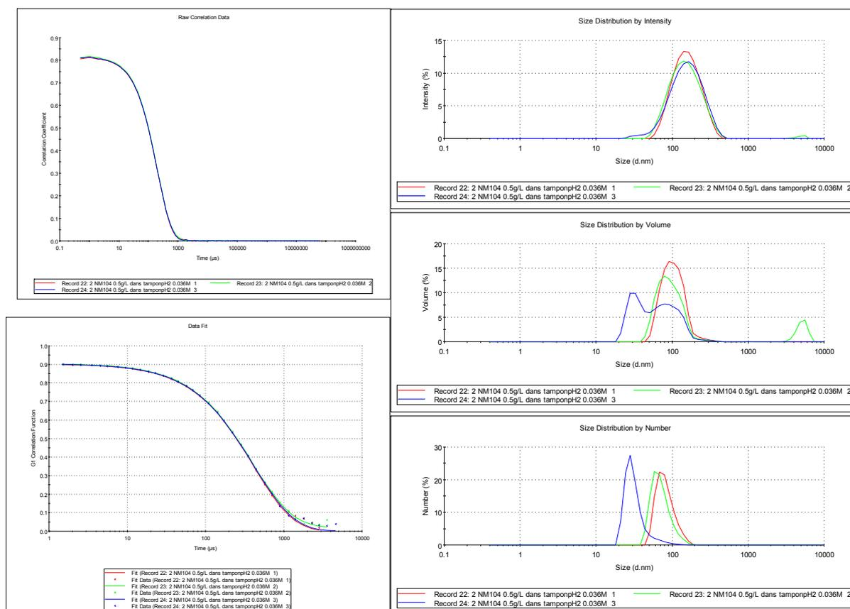
**Figure A9. Main graphs reported by DTS software for 3 consecutive measurements of a NM-104 (TiO<sub>2</sub>) sample (pH 2.8, 0.5 g/L TiO<sub>2</sub> in 0.036 mol/L aqueous ionic medium)**
