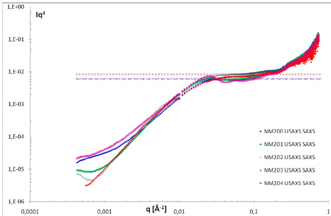
Figure 35. Representation in  $Iq^4$  of SAXS and USAXS results of NM-200 (blue), NM-201 (green), NM-202 (dark blue), NM-203 (red) and NM-204 (pink). The dotted lines are the corresponding Porod's plateaus.
