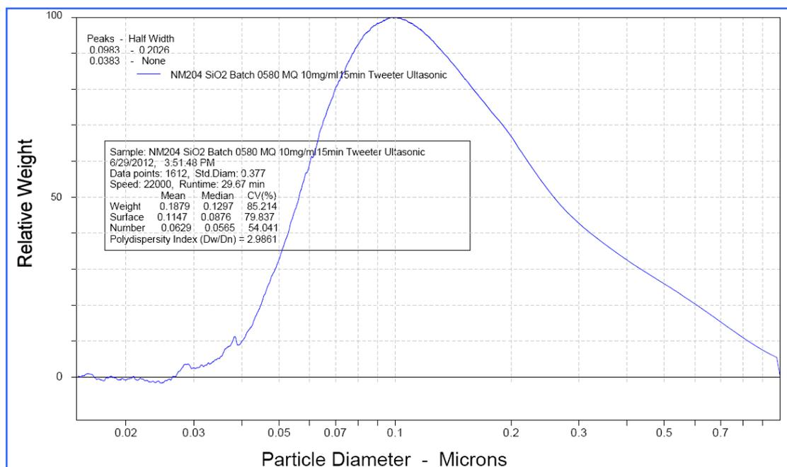
**Figure 31. CLS particle size distribution graph for NM-204.**
