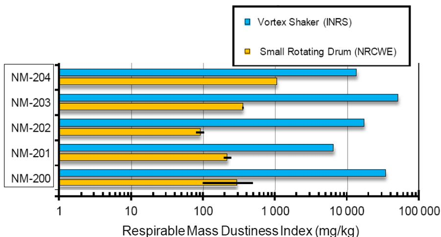
**Figure 77. Comparison between respirable mass dustiness indices obtained with the small rotating drum and vortex shaker method. Errors bars on the SD values correspond to the reproducibility over 3 repeats.**
