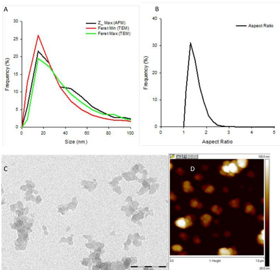
**Figure 67. Characterization of the aggregates of NM-201 in three-dimensions by a combination of TEM and AFM. A) Number based size distributions of Feret Min, Feret max and Z\_max. B) Number based distribution of the aspect ratio. C) Representative TEM and D) AFM micrographs visualizing the morphology of the aggregates.**
