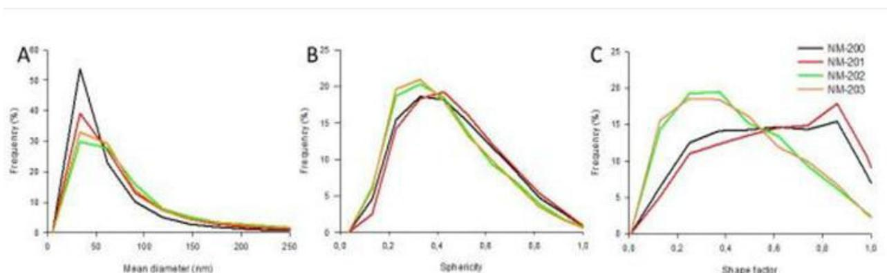
**Figure 64.** Number-based distributions of the mean diameter (A), sphericity (B) and shape factor (C) of agglomerates and aggregates of SAS NMs. The frequency of the agglomerates / aggregates of SAS NM are represented as a function of mean diameter, sphericity and shape factor.
