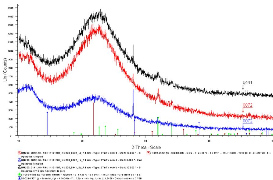
Figure 41. Three XRD scans of NM-200 by NRCWE suggesting presence of Böhmite and  $\text{Na}_2\text{SO}_4$ . Colour code for the X-axis: Böhmite is blue and  $\text{Na}_2\text{SO}_4$  is green. The numbers 0441 and 0072 refer to the vial numbers.
