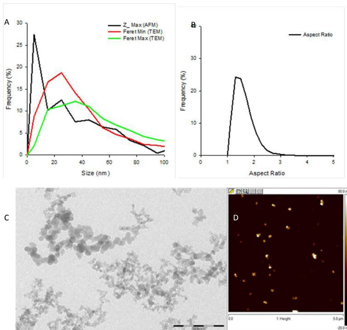
**Figure 69. Characterization of the aggregates of NM-203 in three-dimensions by a combination of TEM and AFM. A) Number based size distributions of Feret Min, Feret max and Z\_max. B) Number based distribution of the aspect ratio. C) Representative TEM and D) AFM micrographs visualizing the morphology of the aggregates.**
