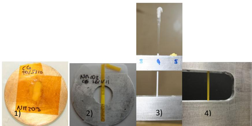
**Figure D2. Examples of different type of cells used for SAXS measurements, 1) double sticky kapton® cell for powders, 2) 1.5 mm flattened polyimide capillary for powders, 3) 1.5 mm glass capillary for powder or liquid samples, 4) 1.5 mm polyimide capillary for powder or liquid samples.**
