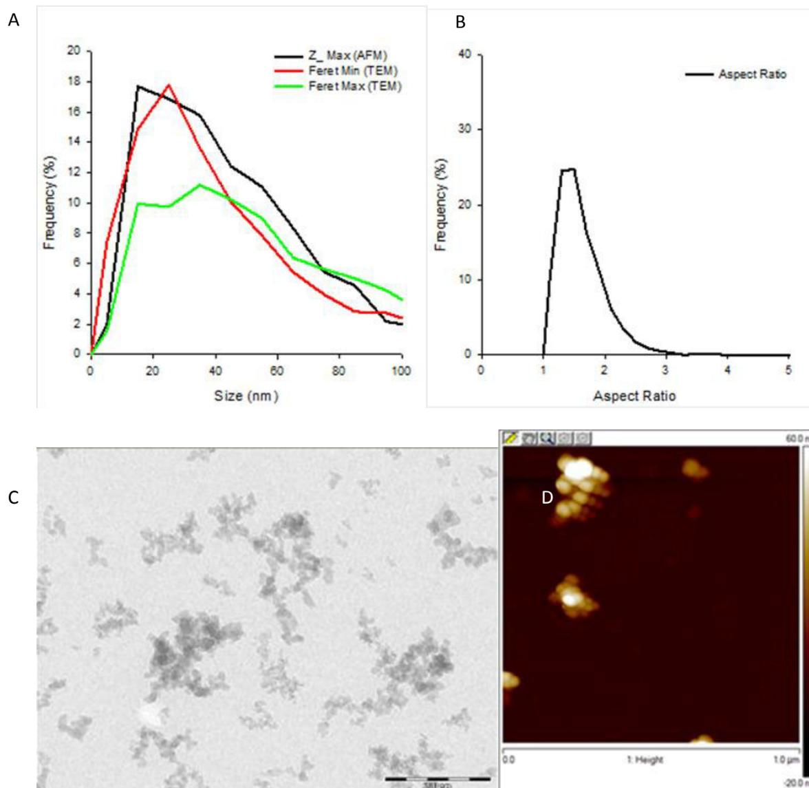
**Figure 68. Characterization of the aggregates of NM-202 in three-dimensions by a combination of TEM and AFM. A) Number based size distributions of Feret Min, Feret max and Z\_max. B) Number based distribution of the aspect ratio. C) Representative TEM and D) AFM micrographs visualizing the morphology of the aggregates.**
