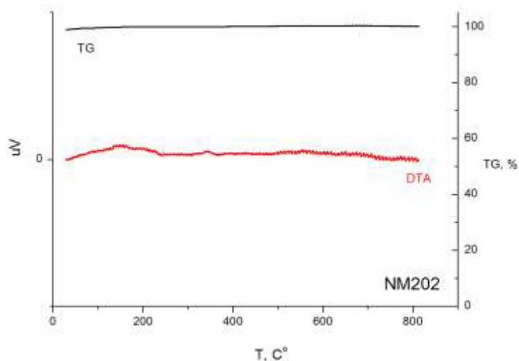
Figure 4. DTA (red curve, unit (left) is  $\mu\text{V}$  [Thermocouple electromotive force]) /TG (black curve, remaining mass in percent (right)) results for NM-202 showing no indication of any phase transformations.
