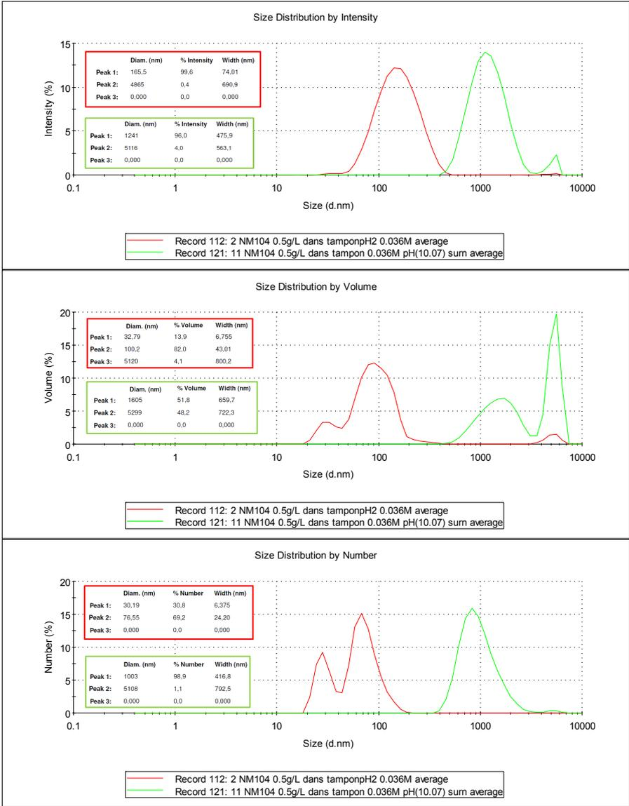
**Figure A8.** Example of size distributions by intensity, by volume and by number, together with tables of numerical values for the three main peaks of each distribution, for two NM-104 (TiO<sub>2</sub>) samples (0.5 g/L TiO<sub>2</sub> in 0.036 mol/L ionic buffer, stable suspension at pH2.8 in red and unstable sample of big aggregates at pH10.1 in green).
