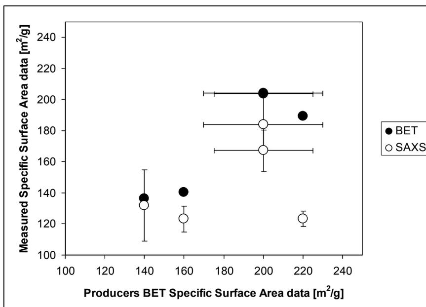
**Figure 38. Plot of measured BET (filled spheres) and SAXS (open spheres) specific surface area data plotted against the BET specific surface area data reported by the producers. Generally, good agreement is observed between measured and producer data. SAXS data appears to underscore the BET surface areas at high surface area values.**
