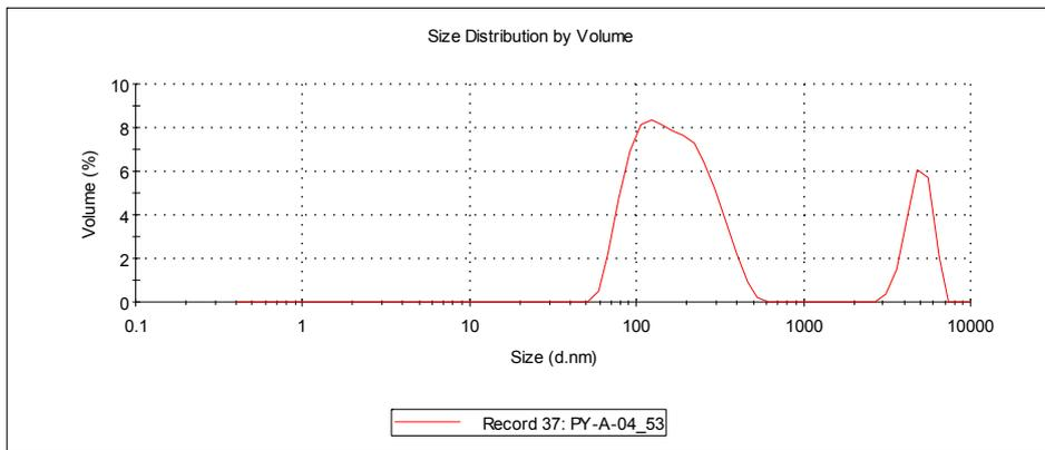
**Figure 24. DLS size distributions for NM-203 dispersed in Milli-Q<sup>®</sup> water. Both the distribution by intensity (top) and the distribution by volume (bottom) are shown. Pdl = 0.184, peak 1 = 186 nm, peak 2 = ~ 2000 nm.**
