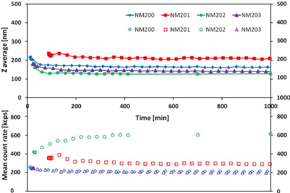
**Figure 21. Evolution of DLS representative quantities (Top: Z-average mean size. Bottom: mean count rate) with residence time over 17 hours for SiO<sub>2</sub> suspensions ultrasonicated (20 min at 40 % amplitude) in pure water.**
