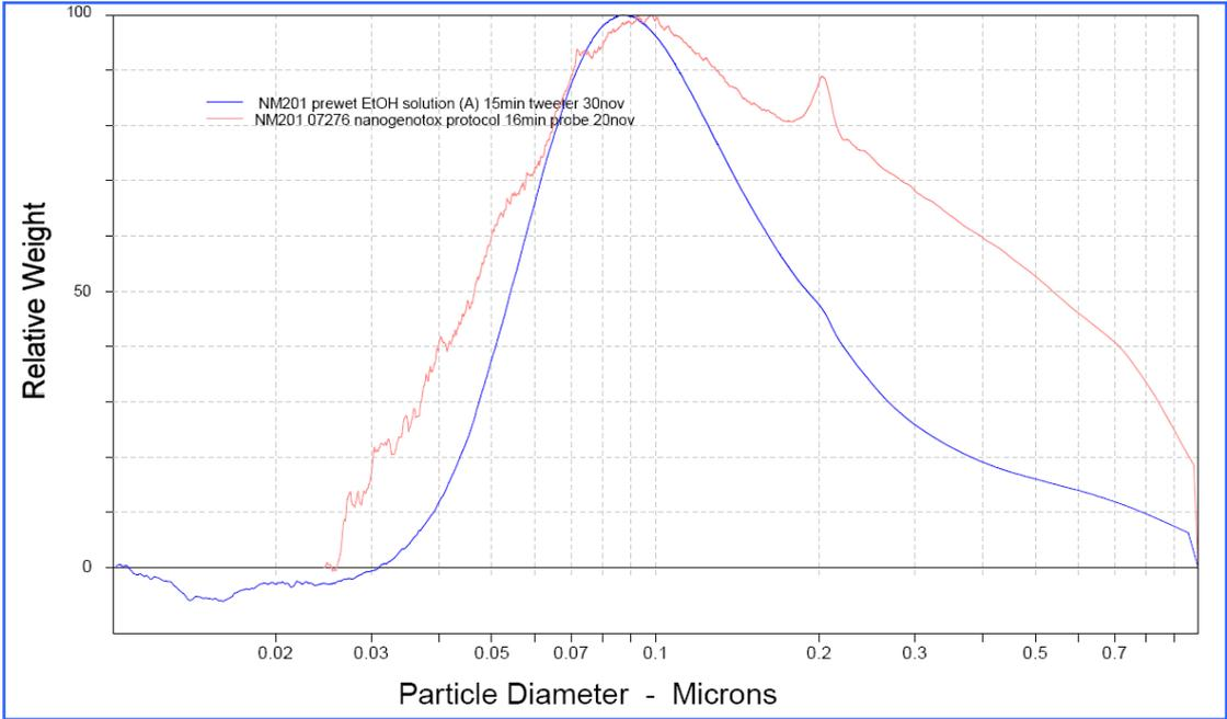
**Figure 28. CLS particle size distribution graph for NM-201.**
