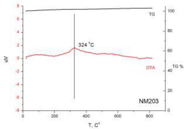
Figure 6. DTA (red curve, unit (left) is  $\mu\text{V}$  [Thermocouple electromotive force]) /TG (black curve, remaining mass in percent (right)) results for sample NM-203. There is a phase transformation at 324 °C.
