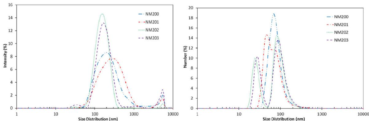
**Figure 22. DLS intensity size distributions (left) and number size distributions (right) for suspensions of SiO<sub>2</sub> nanomaterials dispersed by ultrasonication (20 min at 40 % amplitude) in ultrapure water.**
