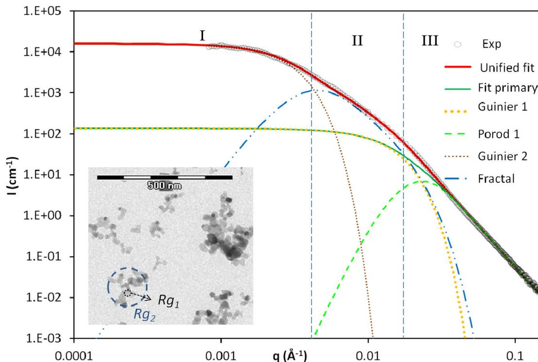
**Figure D6.** Example of SAXS diffractogram (NM-105, a TiO<sub>2</sub>, suspension sonicated at pH 2 as circles) illustrating the unified fit (solid red line) and its components prevailing in each q-domain (dashed-dotted lines). Insert of TEM micrograph (by CODA-CERVA) illustrating the gyration radius of primary particles (Rg1) and aggregates (Rg2) used in the model. Exp = experimental data.
