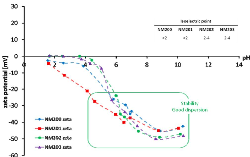
**Figure 32. Zeta potential as a function of pH for SiO<sub>2</sub> NM suspensions (1 g/L) in constant ionic strength aqueous media (0.036 mol/L HNO<sub>3</sub>/NaOH), highlighting the domain of higher stability for pH higher than 5; the IEP values are also reported on the figure.**
