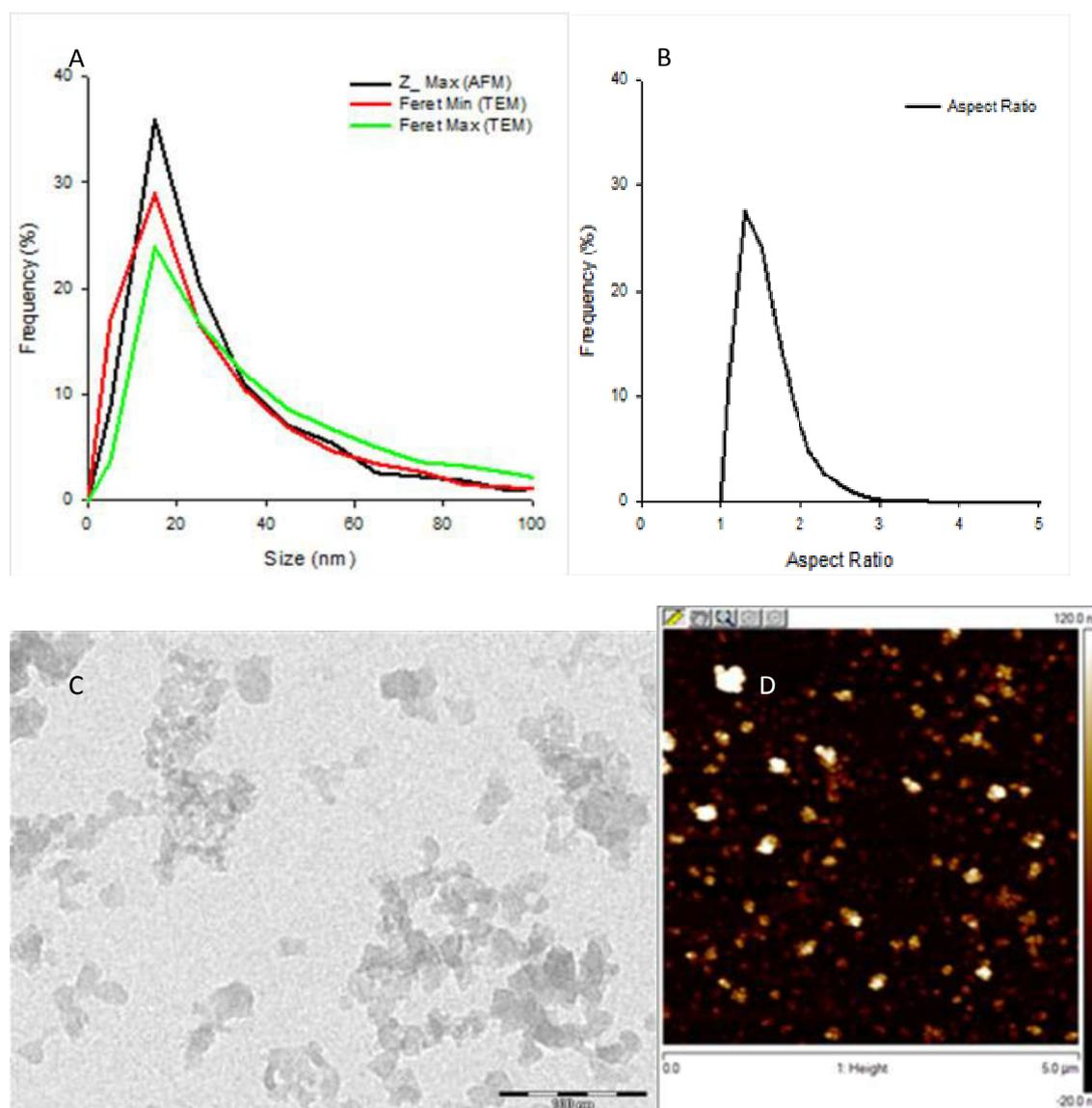
**Figure 66. Characterization of the aggregates of NM-200 in three-dimensions by combination of TEM and AFM. A) Number based size distributions of Feret Min, Feret max and Z\_max. B) Number based distribution of the aspect ratio. C) Representative TEM and D) AFM micrographs visualizing the morphology of the aggregates.**
